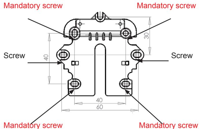
Hold the wall frame against the wall and mark the screw hole positions. Drilling of holes, hole size and the corresponding screws for attaching the panel depend on the wall material.
