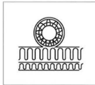
Duct insulation, alt. A
