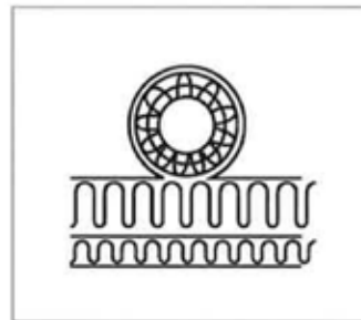
Duct insulation, alt. A
